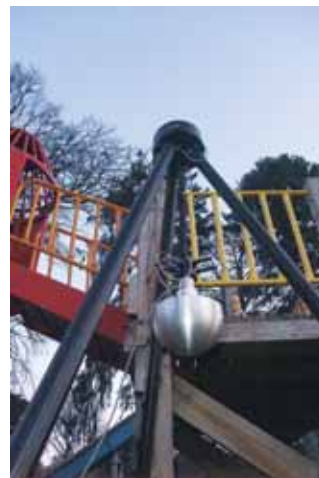
Testing playground matting for free fall height safety
